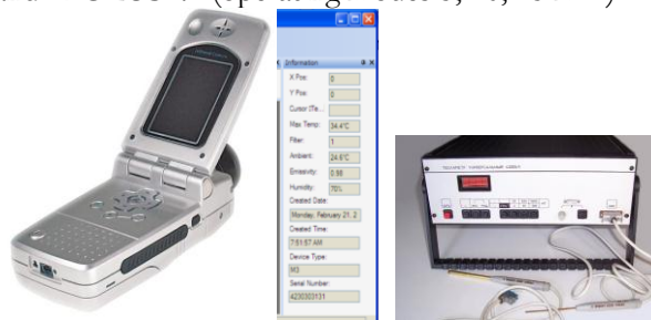
Fig. 5. The infrared camera "MobiR M3", the temperature informational table and the universal teslameter 43205.
